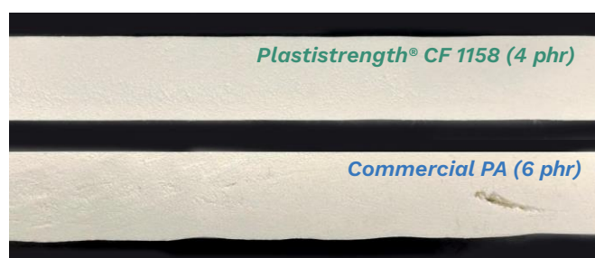
Figure 2: The cell structure and surface finish in rigid PVC foamed sheet made with Plastistrength® CF 1158 process aid (top), and a typical commercial process aid (bottom)
