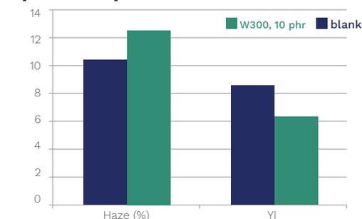
Formulation (phr): PVC Kw62: 100, tin maleate: 2.1, internal lubricant: 0.8, ESBO: 1, Plastistrength® 550 PA: 2, Plastistrength® L1000 PA: 0.15, oxidised PE wax: 0.15, UVA: 0.3
