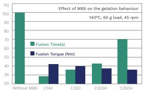
Typical calendering formulation (phr): PVC Kw57: 100, Octyl Organotin Stabilizer: 1.2, internal lubricant: 0.8, ESBO: 1, Plastistrength® 550 process aid: 1, Plastistrength® 770 process aid: 0.7, Clearstrength® C impact modifier: 9
